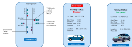
Enforcement Officer visits red icons and confirms their ID using wireless validation (Bluetooth Low Energy)
